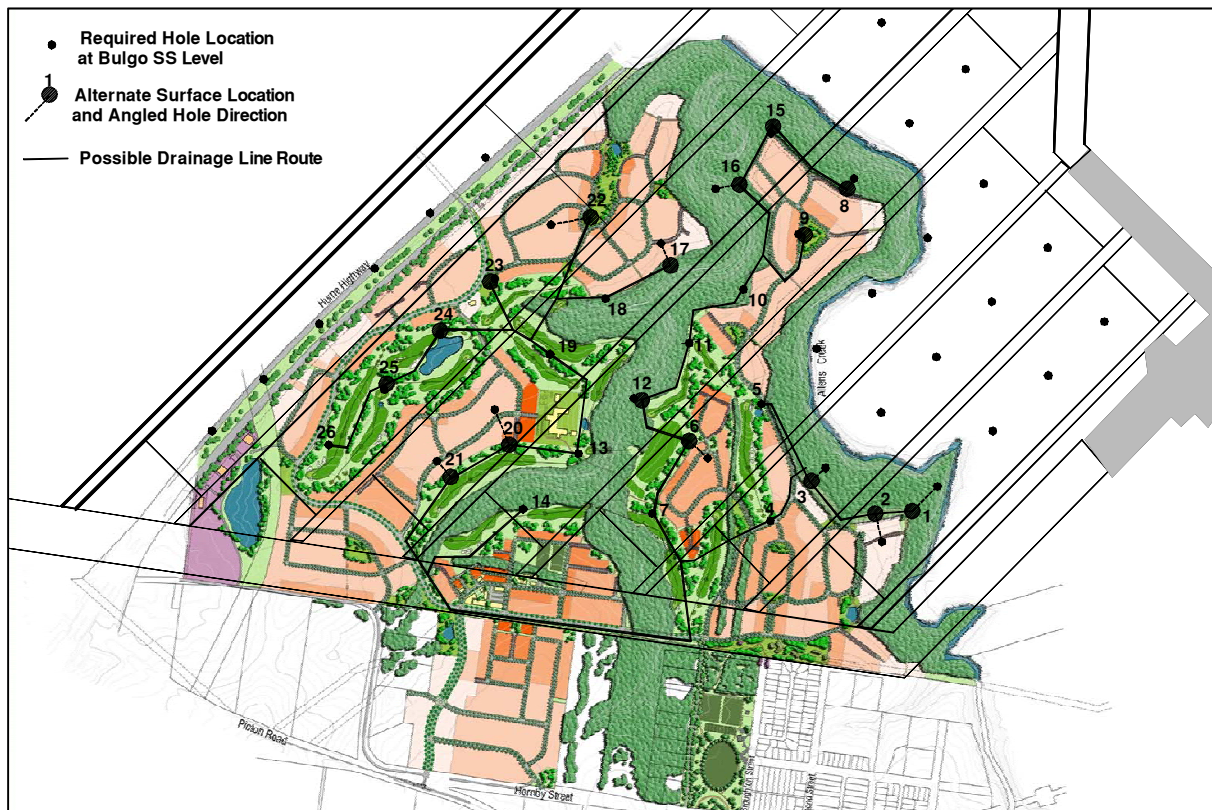
Figure 26 : Proposed Bingara Gorge Gas Drainage Layout (IMC, 2003)
